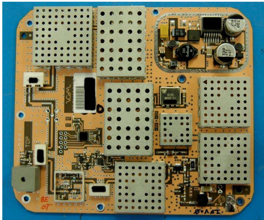
**13.11 TR2525B – Board with shield off**
