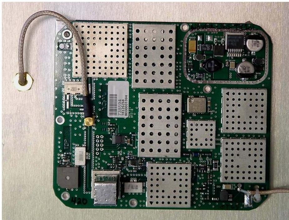
**13.15 TRI2525B – Board with shield off**
