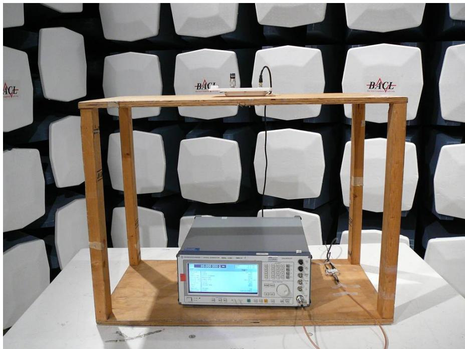
**12.4 Transmitter Radiated Emission – Rear View (TR2525B)**
