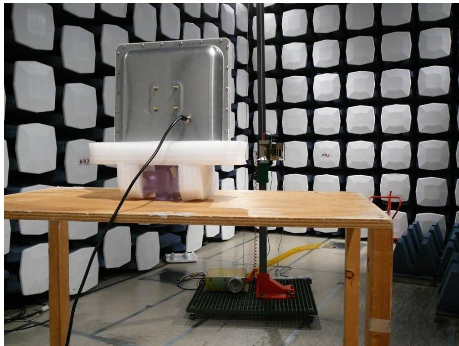
**12.3 Transmitter Radiated Emission – Front View (Model: TR2525B)**
