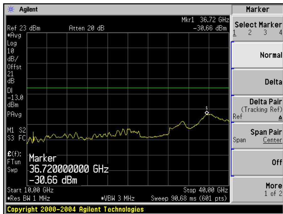
**Channel Bandwidth = 7.0 MHz, Low Channel****30 MHz – 1 GHz**
