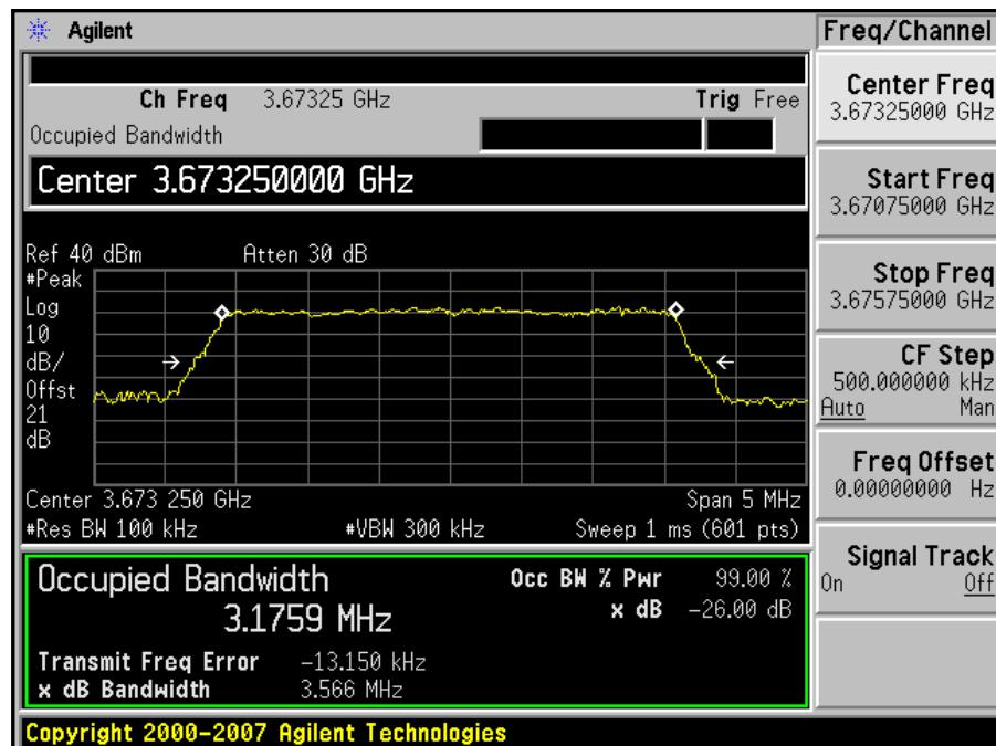
**Channel Bandwidth = 7.0 MHz****Low Channel (Fc = 3653.50 MHz)**
