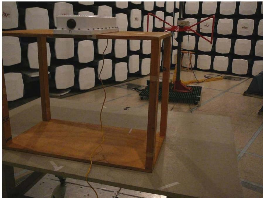
**Radiated Emission above 1 GHz Back View**
