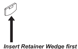
Figure A-3 Placing the Molex Backshell on
