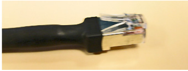
Figure A-10 Connector wrapped in ZTHS.50-01 sheath
