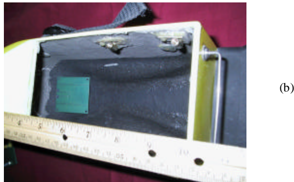
Figure 5. (a.). Location of the internal antenna shown from the outside of the case. (b). Location of the internal antenna with the camera electronics removed. The distance from the antenna to the user exceeds the minimum 20 cm necessary for mobile devices.
