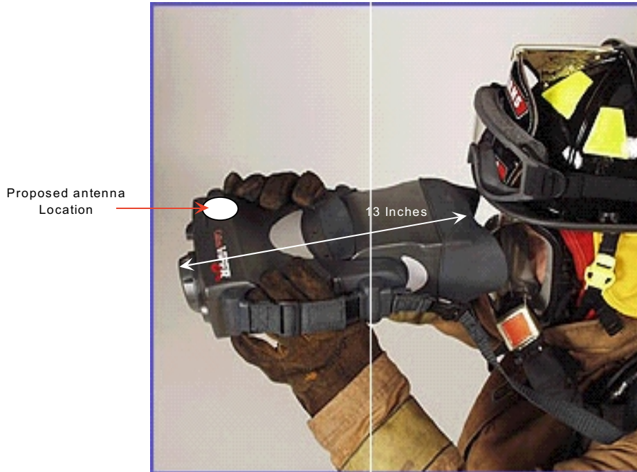
Figure 3. Figure of the external camera. Internal photos are confidential. Note that the antenna will be placed at a sufficient distance away from the body.
