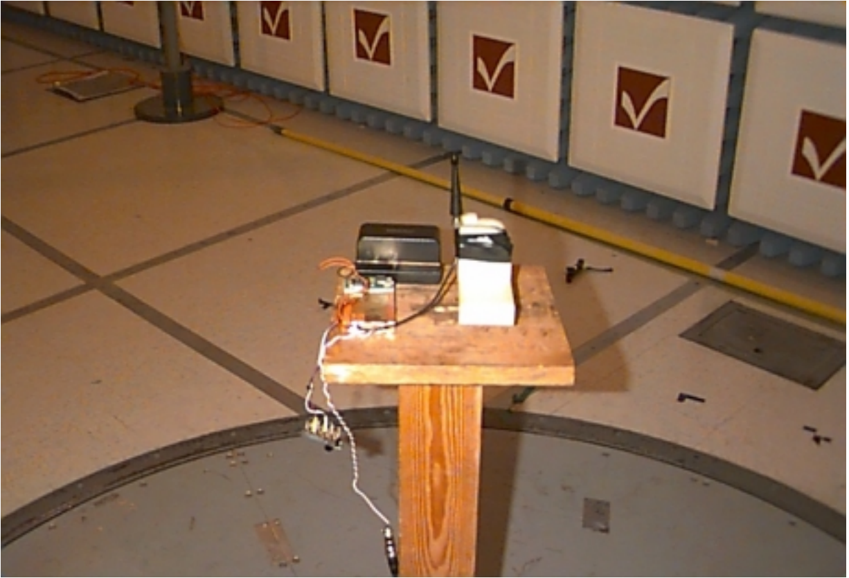
View of the K & A Wireless model VTRAN-2500 module during the Radiated Emissions tests.
