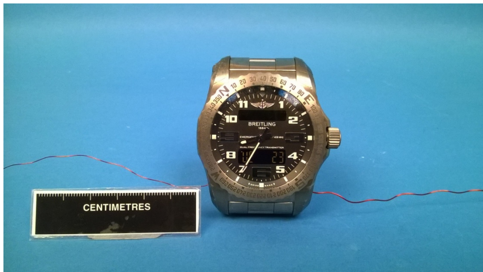
Radiated Sample (antennae deployed)
