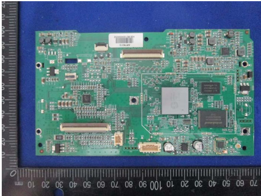
EUT – Main Board Top Uncover View
