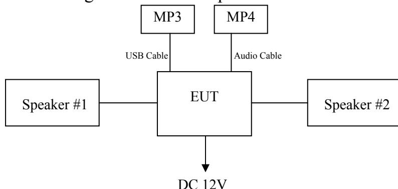
(EUT: Marine Audio System with AM/FM/WB/USB-ipod/Aux in/Bluetooth)
