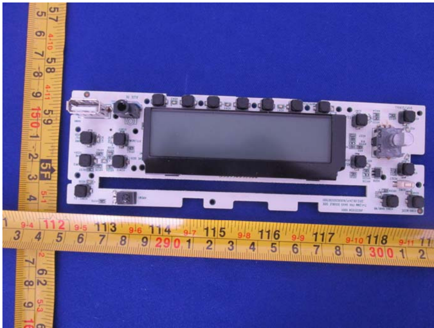
EUT –Panel Board Top View
