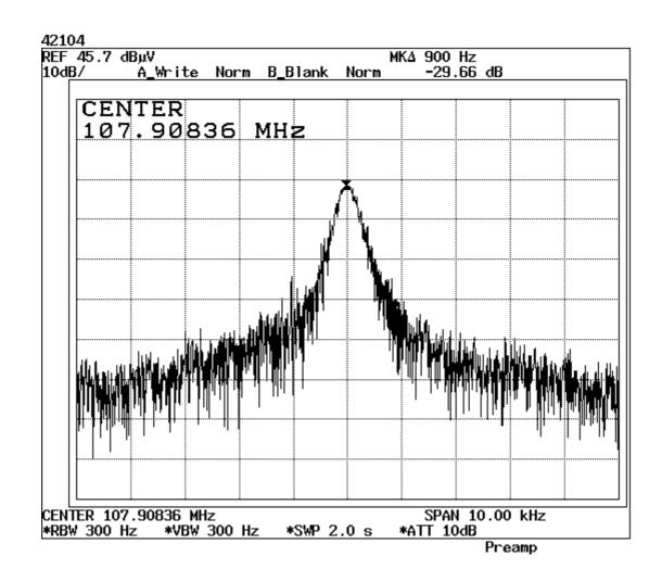
Result : The field strength of any emission within the operation band did not exceed 48  $dB(\mu V/m)$  for average value or 68  $dB(\mu V/m)$  for peak value. Refer to page 9 for the recorded value for the emission at the fundamental frequency.
