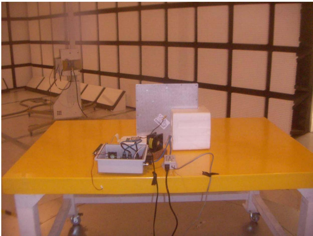
**RADIATED RF MEASUREMENT SETUP, FRONT VIEW**
