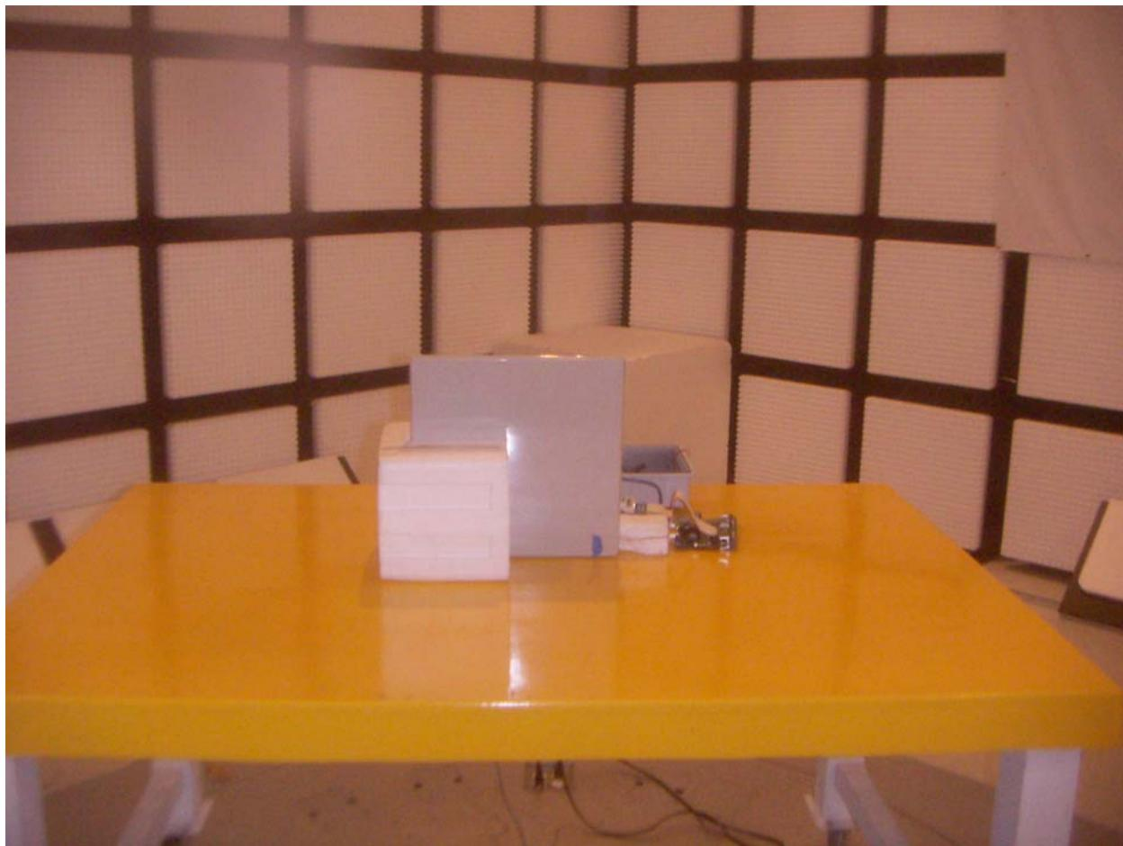
**RADIATED TEST SET-UP, EUT CLOSEUP**
