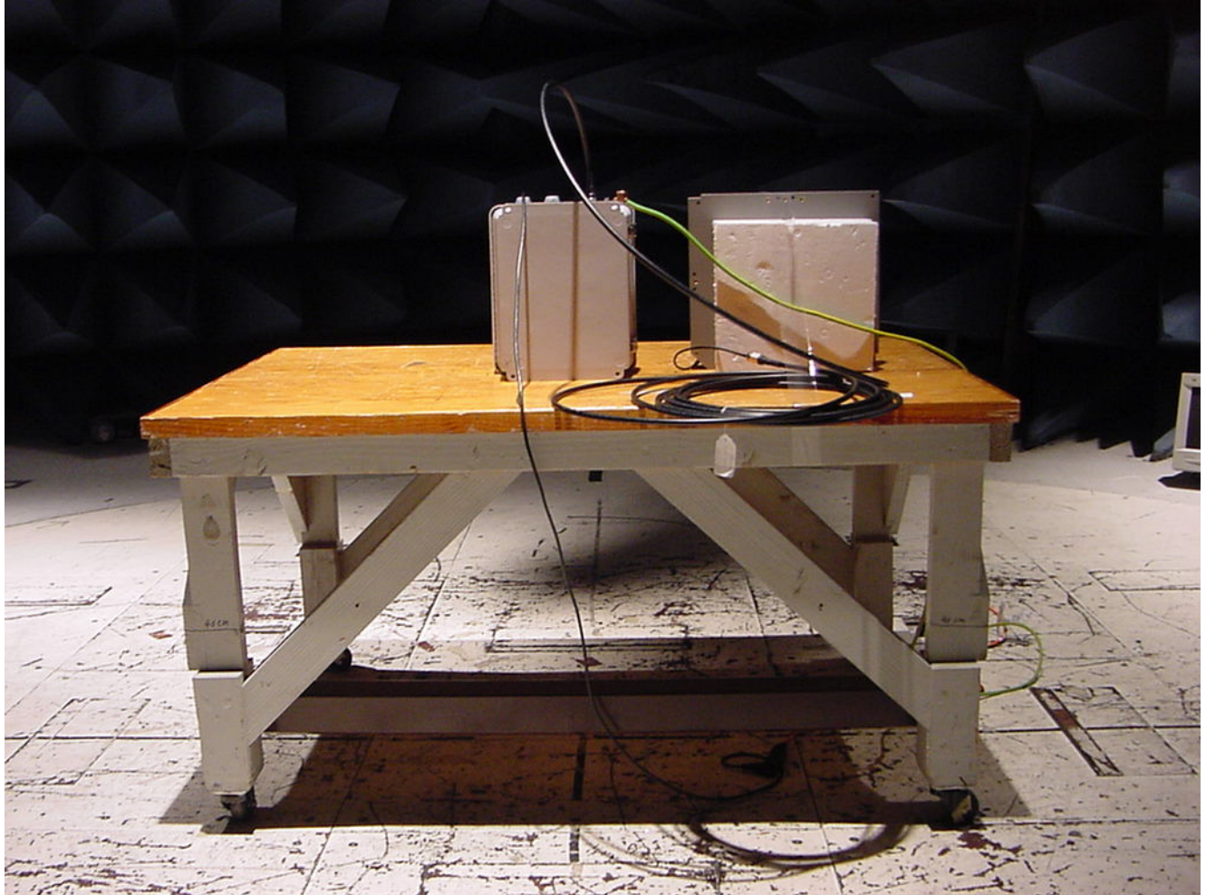
Photograph 7. Radiated Emission Limits TB 2.4-5.8 (2400-2483.5 MHz) Test Setup
