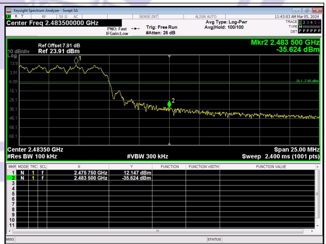
Out Of Band Emission(Right) FSK_Channel Hopping
