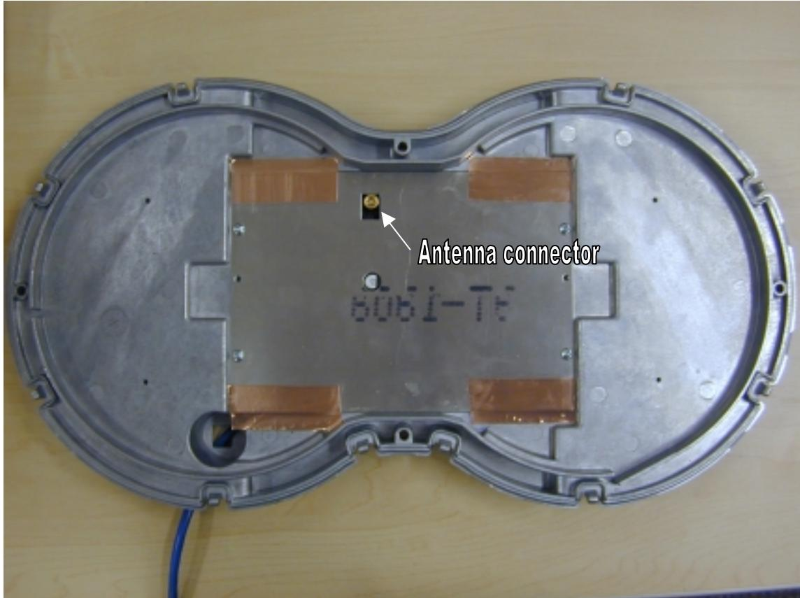
The following picture shows the bottom side of the antenna with the double-sided tape that is used to secure the antenna to the chassis in three locations. The double-sided tape is Rogers Corp. Poron 4790-92-15250-04 with 3M 468MP adhesive on both sides.
