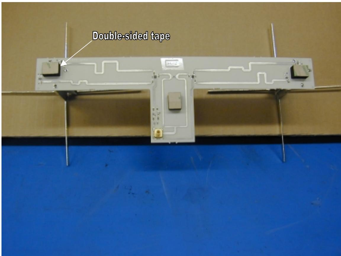
The following picture shows the antenna assembled on the modem card. Note that if the antenna is removed from the chassis, the double-sided tape will tear and the antenna cannot be securely installed again.
