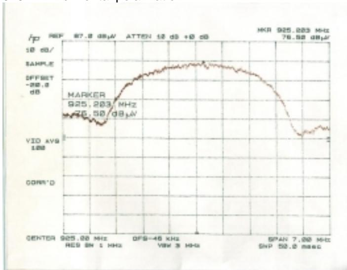
The power under the curve was integrated in 1MHz bins and correction factors applied to account for cable loss and path loss giving the following results. Note that the power at the antenna port was calculated from the EIRP measurements assuming an antenna gain of 10.2dB in vertical polarization and 8.2dB in horizontal polarization.
