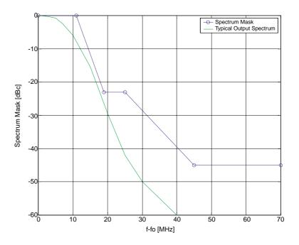
*Figure 10–1 Transmitter Mask*
