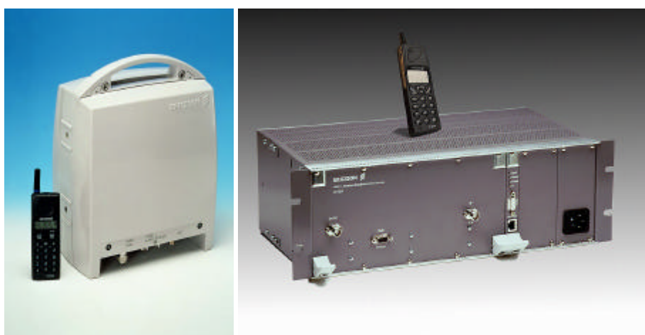
Figure 10. The prototype version of the Access Termination: the User Radio Unit, the antenna and the Network Unit.
