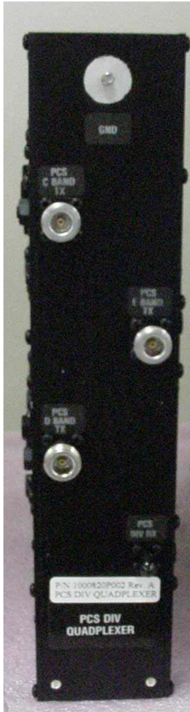
Figure 7-5 Quadplexer, PCS Diversity (Transmitting Blocks C/D/E)
