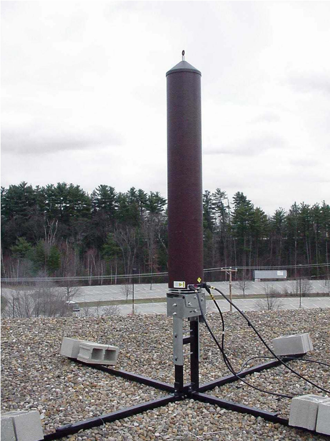
Figure 6-5 RAN Antenna (Polarization Diversity Version)
