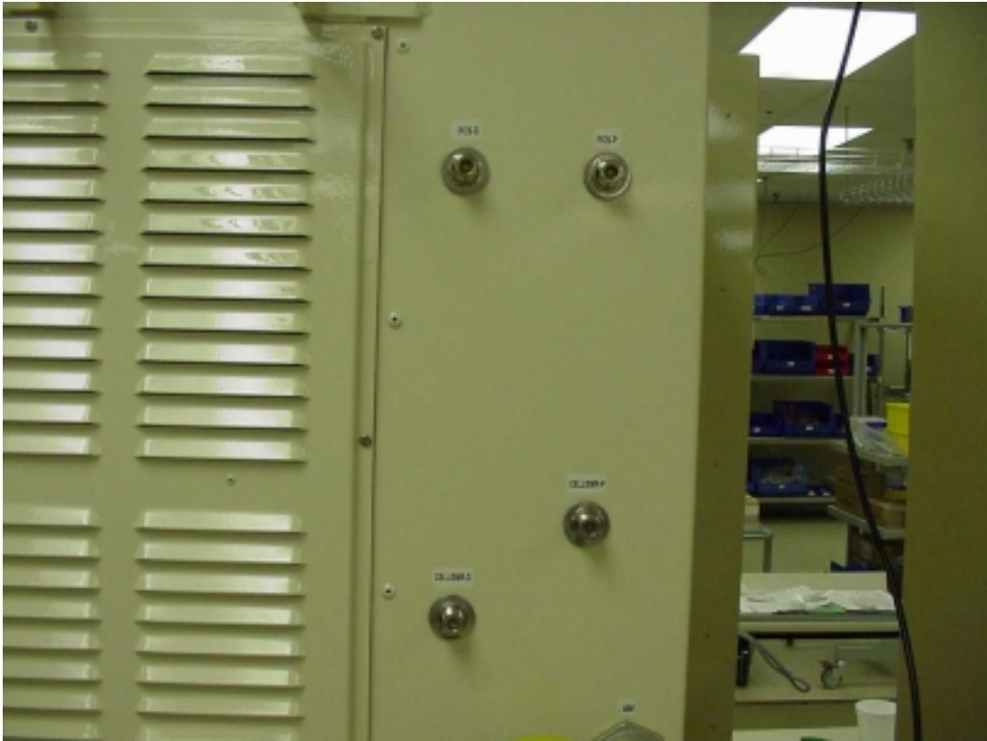
Figure 6-3 Detail of RF Connector Identification on Rear of RAN
