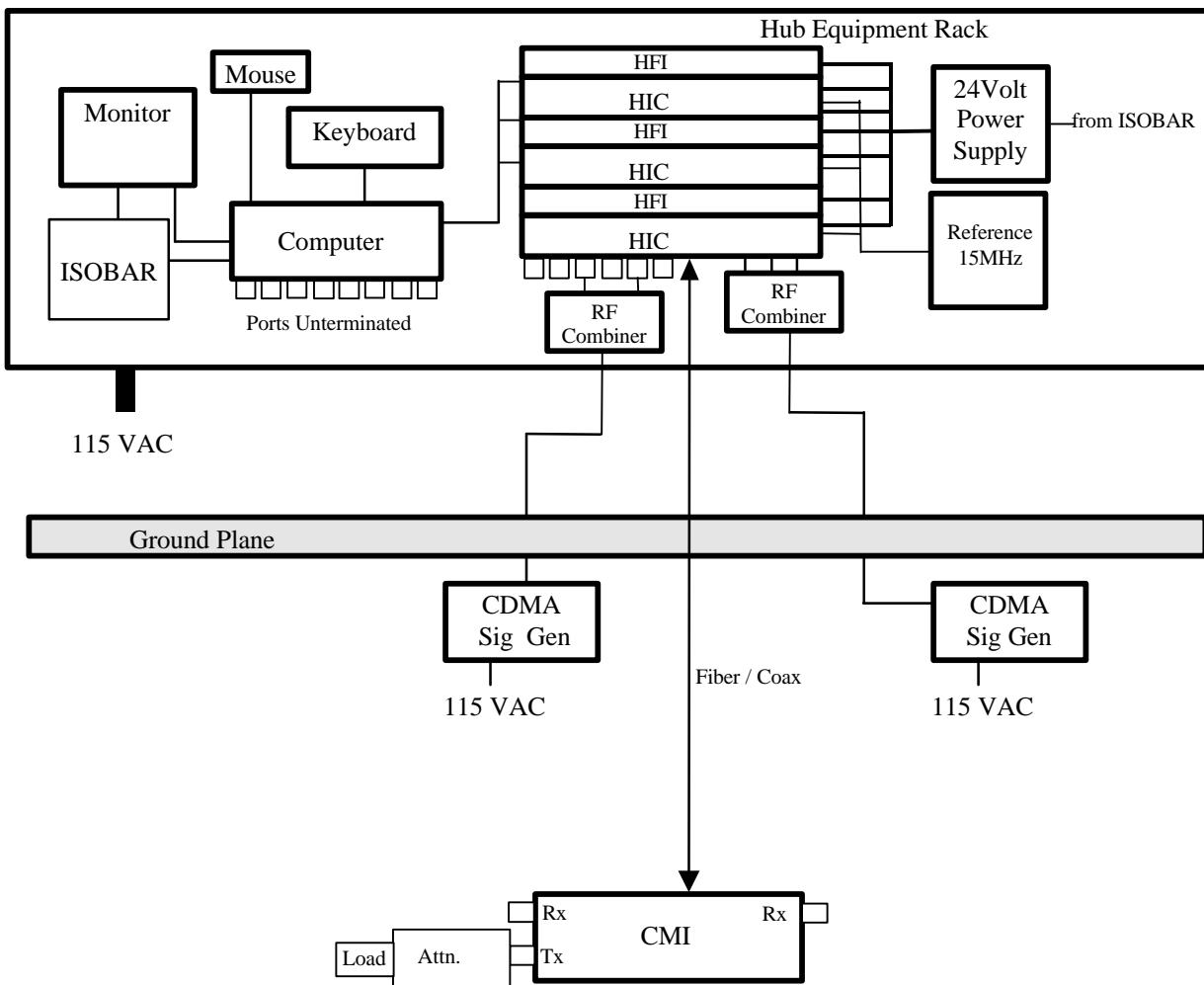
**Figure 3-2 Hub Equipment Rack Radiated Emissions Test Setup**
