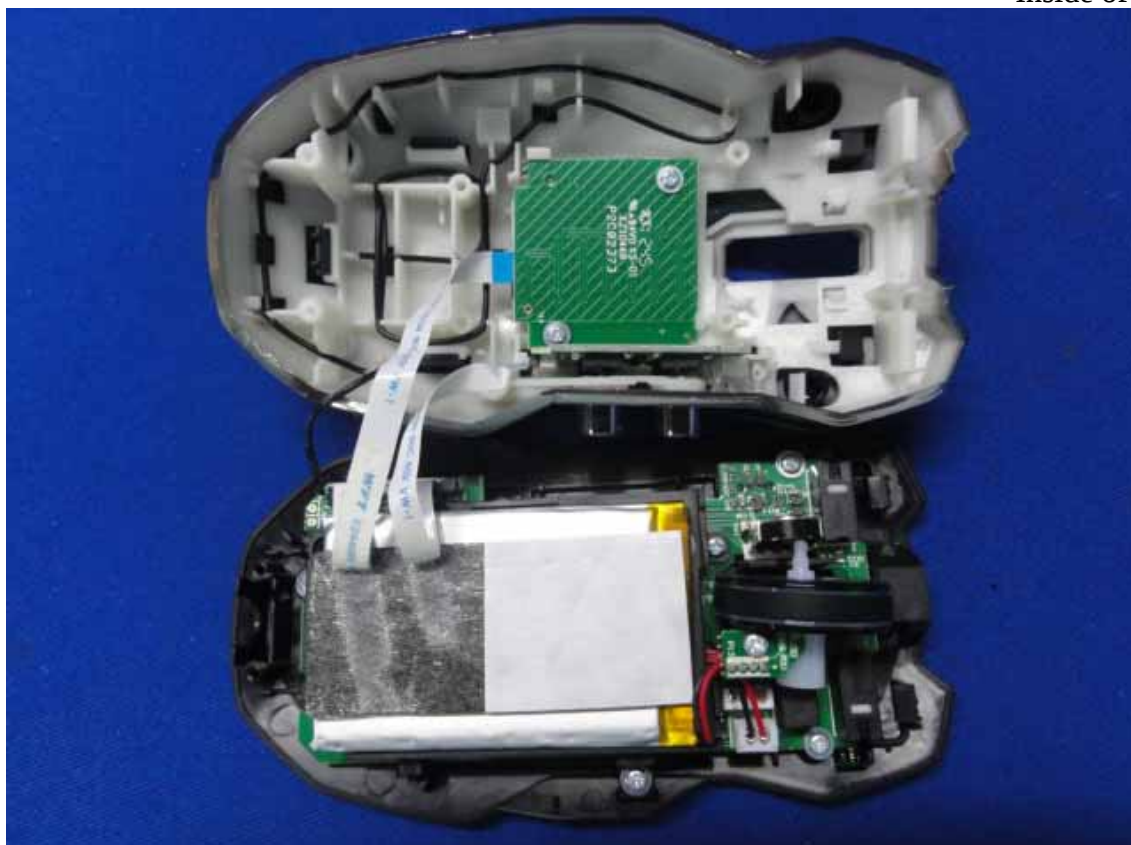
Figure 6 Inside of the EUT
