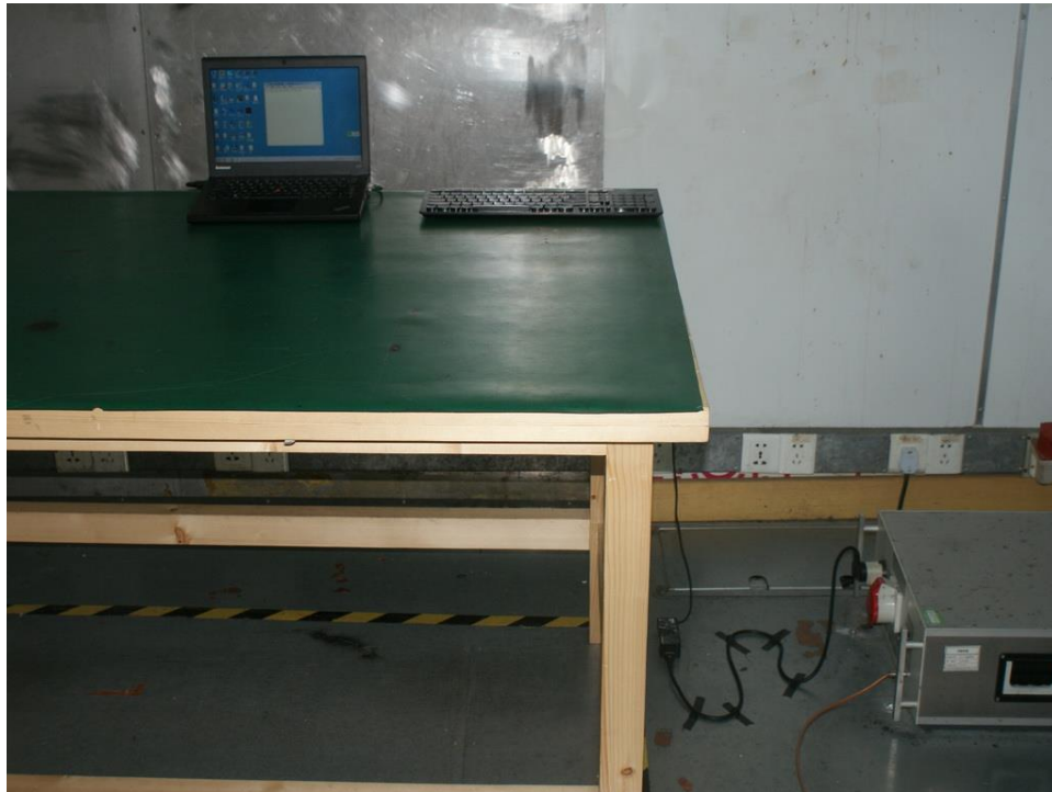
Photograph 1: Set-up for Conducted Emission
