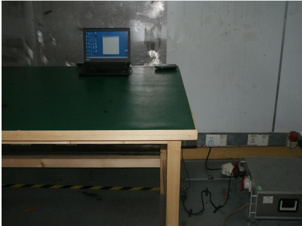
Photograph 6: Set-up for Radiated Emission (30MHz ~ 1GHz)
