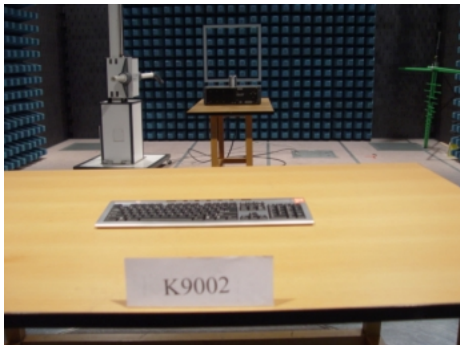
Photograph 1: Set-up for Radiation Measurement Below 30MHz
