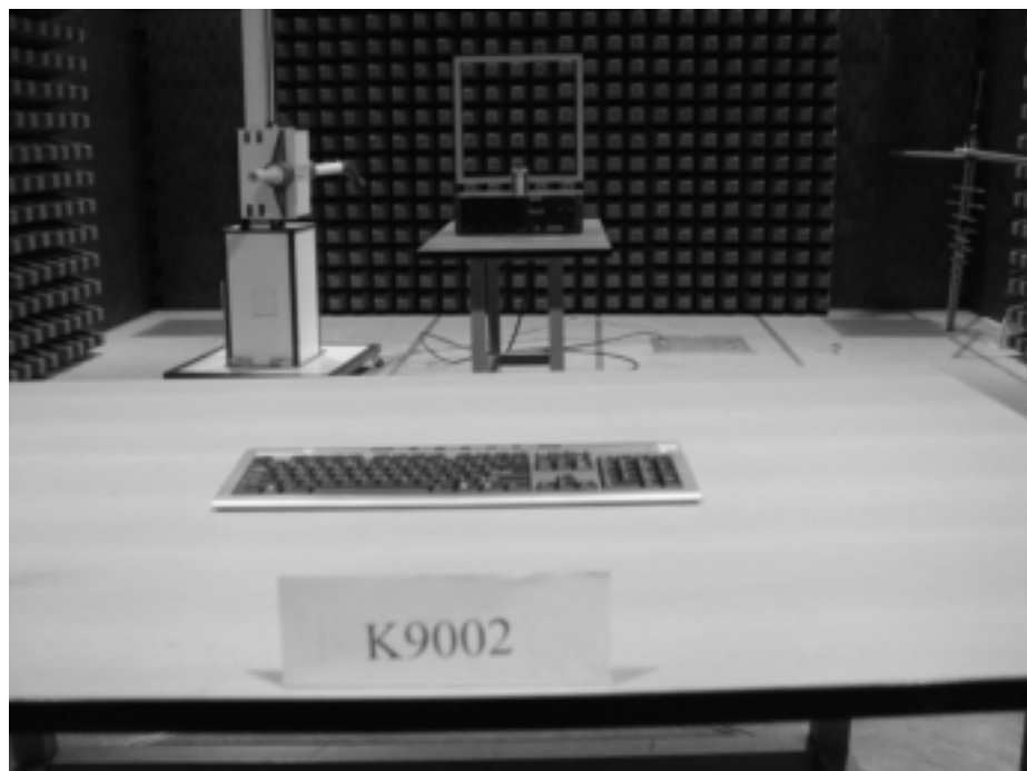
Photograph 1: Set-up for Radiation Measurement Below 30MHz
