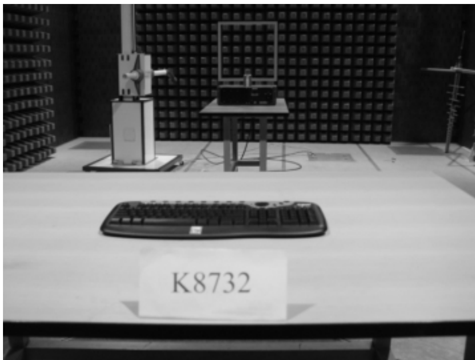
Photograph 1: Set-up for Radiation Measurement Below 30MHz
