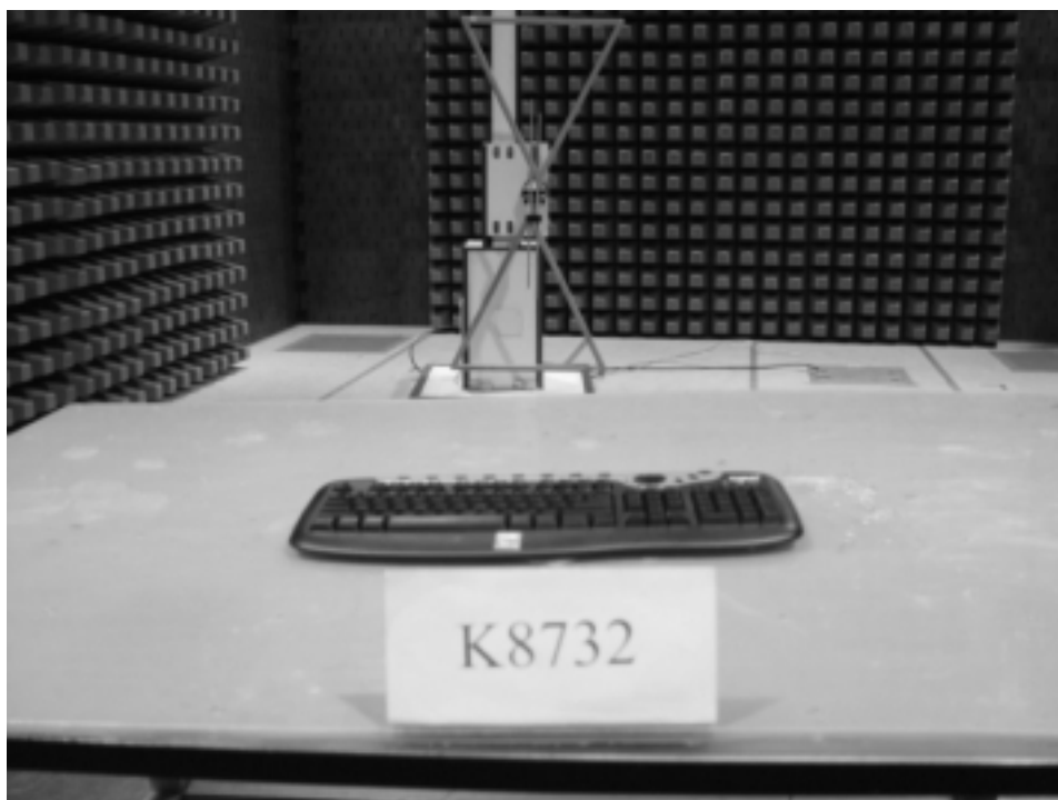
Photograph 2: Set-up for Radiation Measurement below 1GHz
