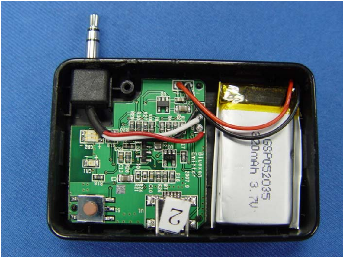
Figure 8 Component Side of the PCB
