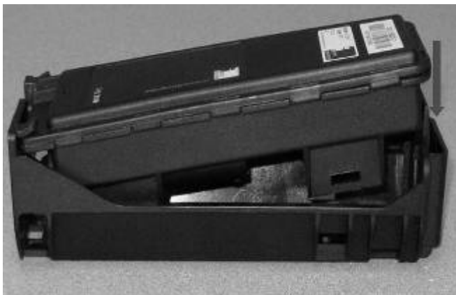
Figure 4.2 Installing the SET transponder into the bracket
