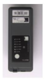
The i-Q310 series of tags is IDENTEC SOLUTIONS' well-established generation of Intelligent Long Range® (ILR®) active RFID tags based on the ISO 18000-7 standard.
