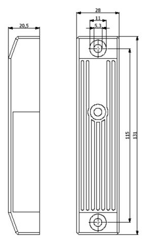
All dimensions in mm. External cable to temperature sensor (models i-Q350T & i-Q350TL) not shown.
