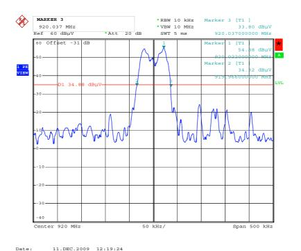
Permitted frequency band: 902 - 928 MHz 20 dB bandwidth: 71.0 kHz Carrier frequency stability: specified Maximum frequency tolerances: Bandwidth of the emission: 71.0 kHz within permitted frequency band<sup>6</sup>:  $\boxtimes$  yes no no
