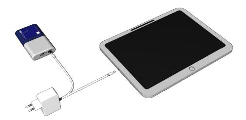
The DC power plug can be used when a permanent connection is required. For instance can the plug be used to share a power supply for simultaneous charging a tablet pc and the reader. The connected reader will remain IP65 rates as the DC power supply plug sealed. Removing the rubber USB protection plug and connecting USB will reduce the IP rating to IP52.
