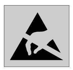
This product contains components that are sensitive to electrostatic discharges. Please observe the special instructions for their protection. Incorrect handling can damage the unit and cause the invalidation of the warranty.
