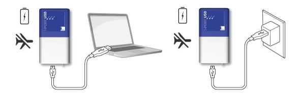
Both connection methods will also charge the internal battery.
