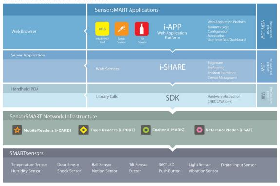
The SensorSMART Platform infrastructure features mobile readers (i-CARD), fixed readers (i-PORT) and exciters (i-MARK). Network sensors offer the highest functionality within the SensorSMART Platform. Robust and reliable, SMARTsensors monitor temperature, humidity, light, shock, tilt, motion, push button, digital input, Hall sensor, etc.
