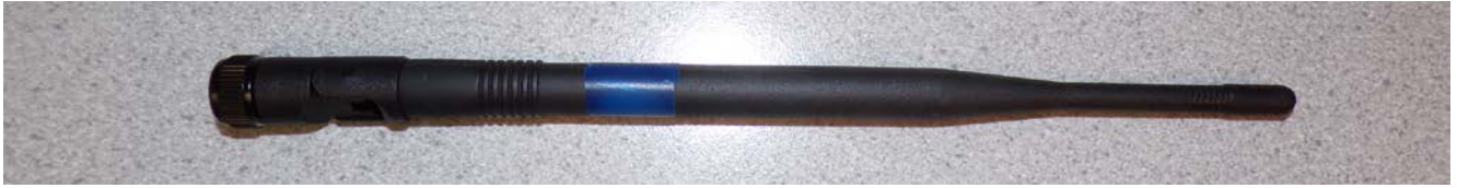
Antenna type 1: 289070 ILR – half-wave dipole antenna SMA i-CTA868 MH (2dBi)
