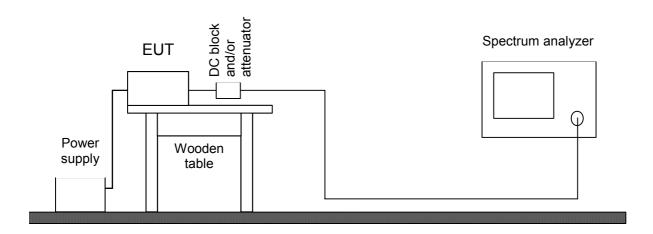
Test instruments used for conducted measurements:
