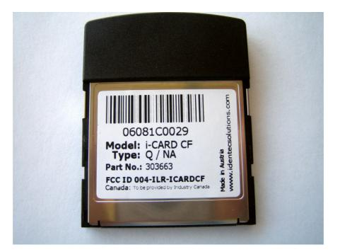
The i-CARD CF carries it's type label on the back side of the CF card.
