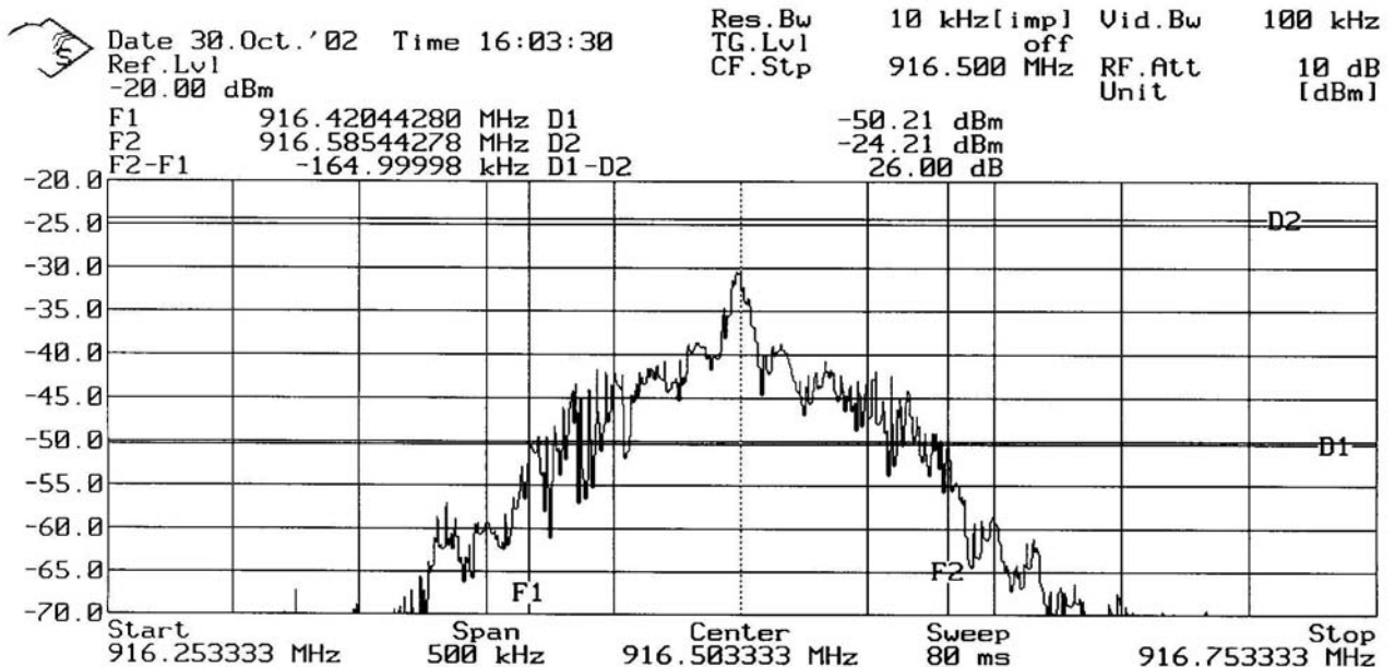
Plot 1.2: EUT: i-Card3 connected via RS232 port to laptop PC; 26 dB Bandwidth (normal operating mode: continuous tag reading process, 0.1 s delay)
