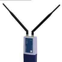
The i-PORT M352 UHF is used as a reader in Identec's system.
