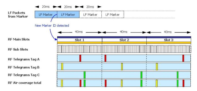
The last row shows how the random use of the timeslot avoids collision between the tags.
