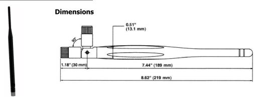
Half-wave Dipole Antenna Ordering number:
