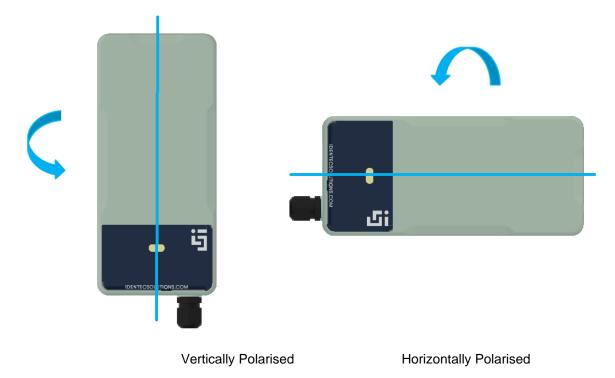
Polarization is dependent on orientation and is rotation symmetrical.
