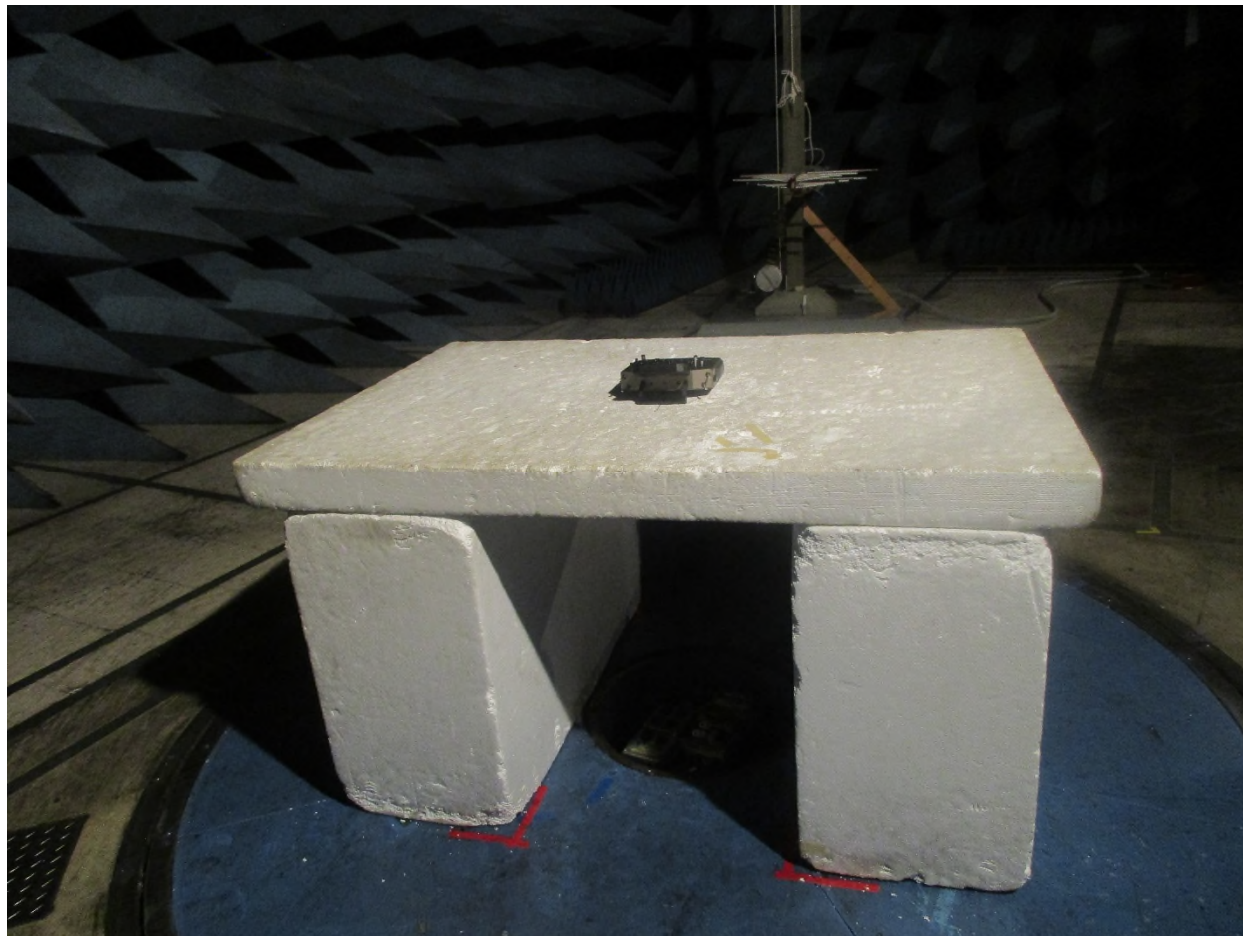
Figure 4: Radiated Emissions – Back View – 200 MHz – 1 GHz – EUT Flat
