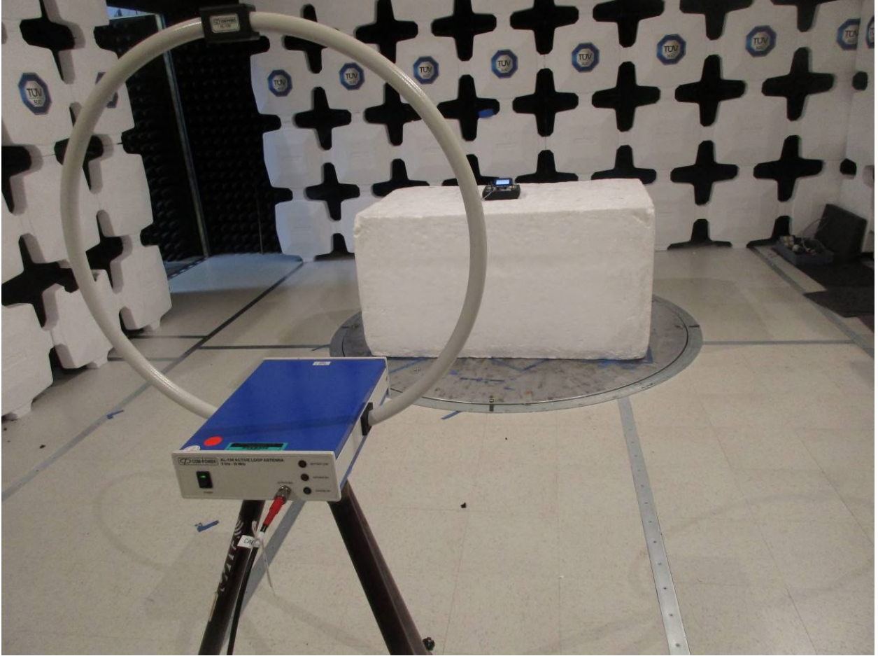
Figure 7: Radiated Emissions – Front View - Below 30 MHz - EUT Flat
