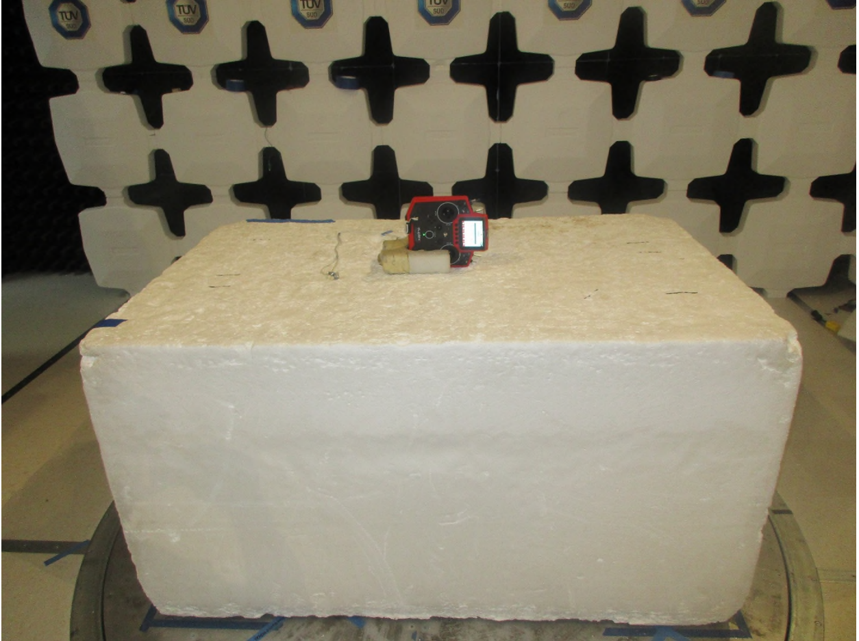
Figure 6: Radiated Emissions – Front View – below 1 GHz – EUT on Side
