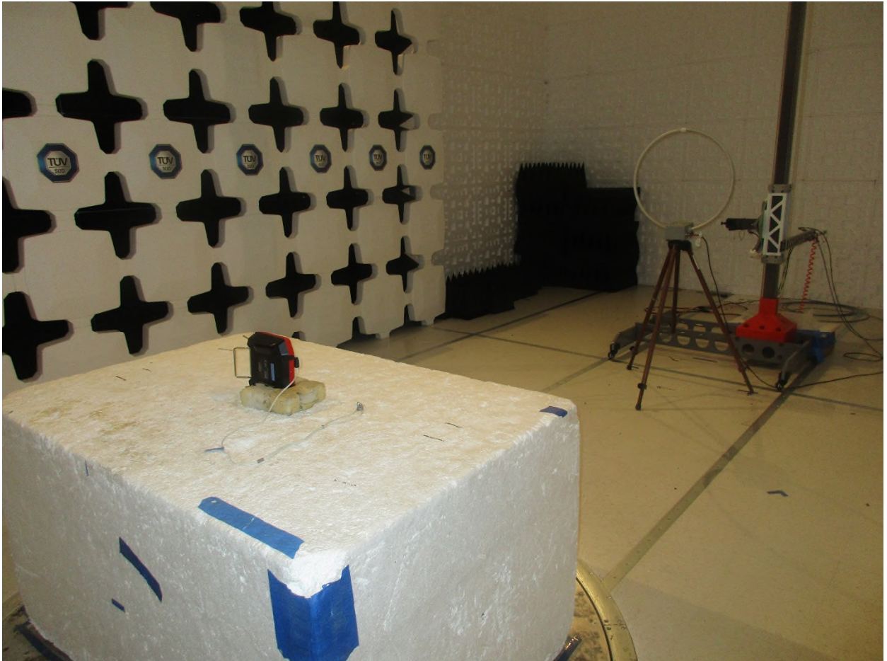
Figure 7: Radiated Emissions – Back View – 9 kHz -30 MHz – EUT on Side
