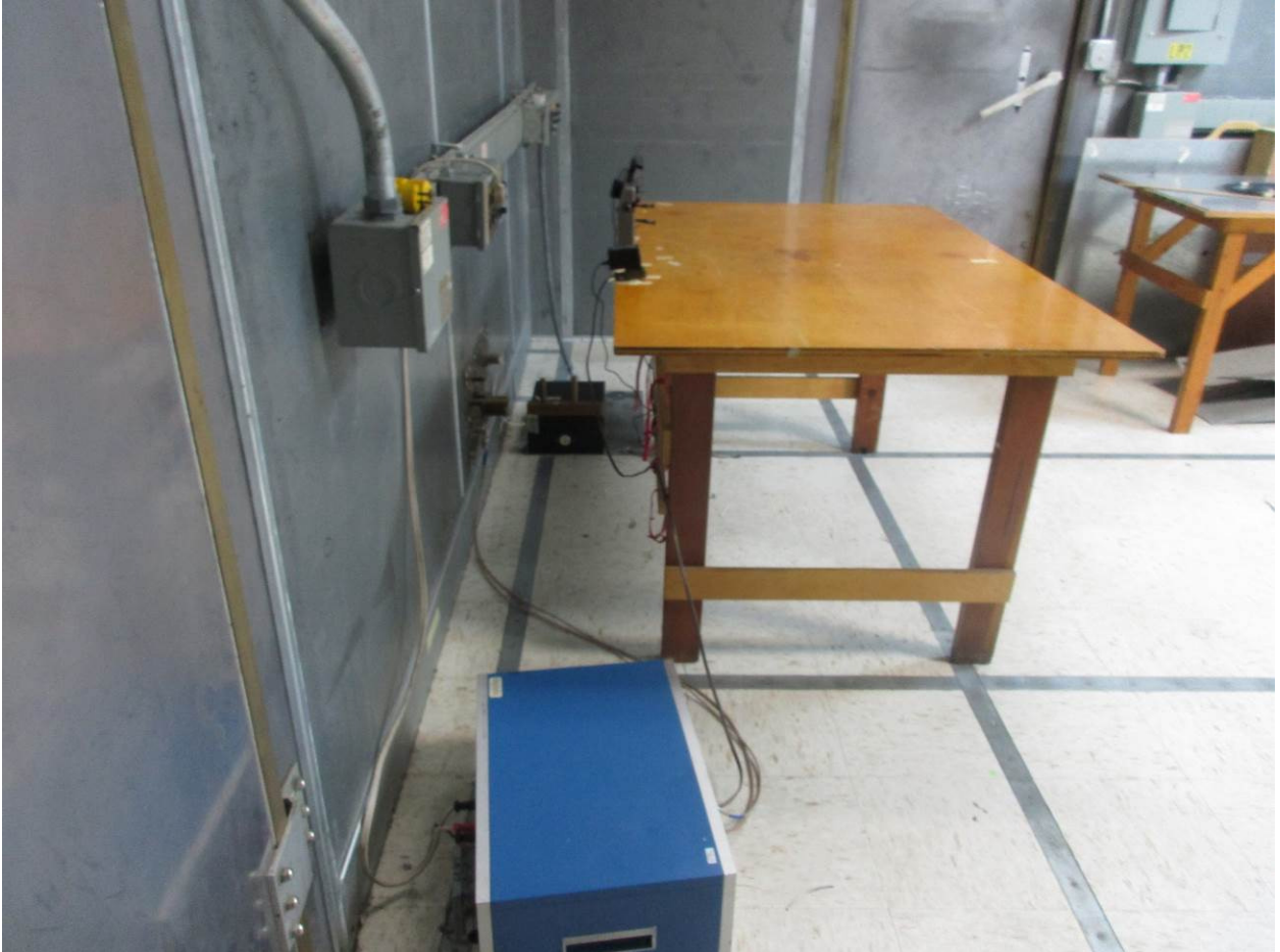
Figure 17: Power Line Conducted Emissions – Side View
