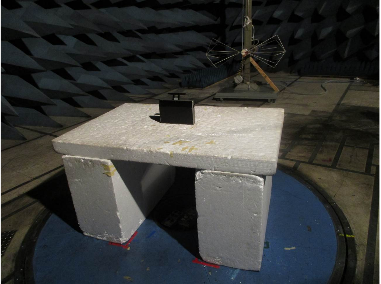
Figure 3: Radiated Emissions – Back View – 30 MHz – 200 MHz (900 MHz)
