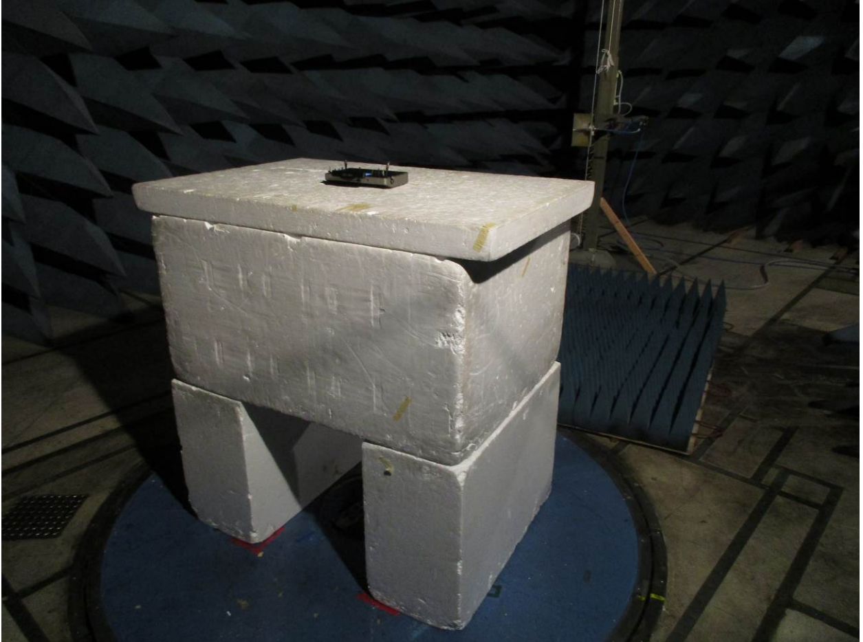
Figure 12: Radiated Emissions – Back View – Above 1 GHz (2.4 GHz Spurious)
