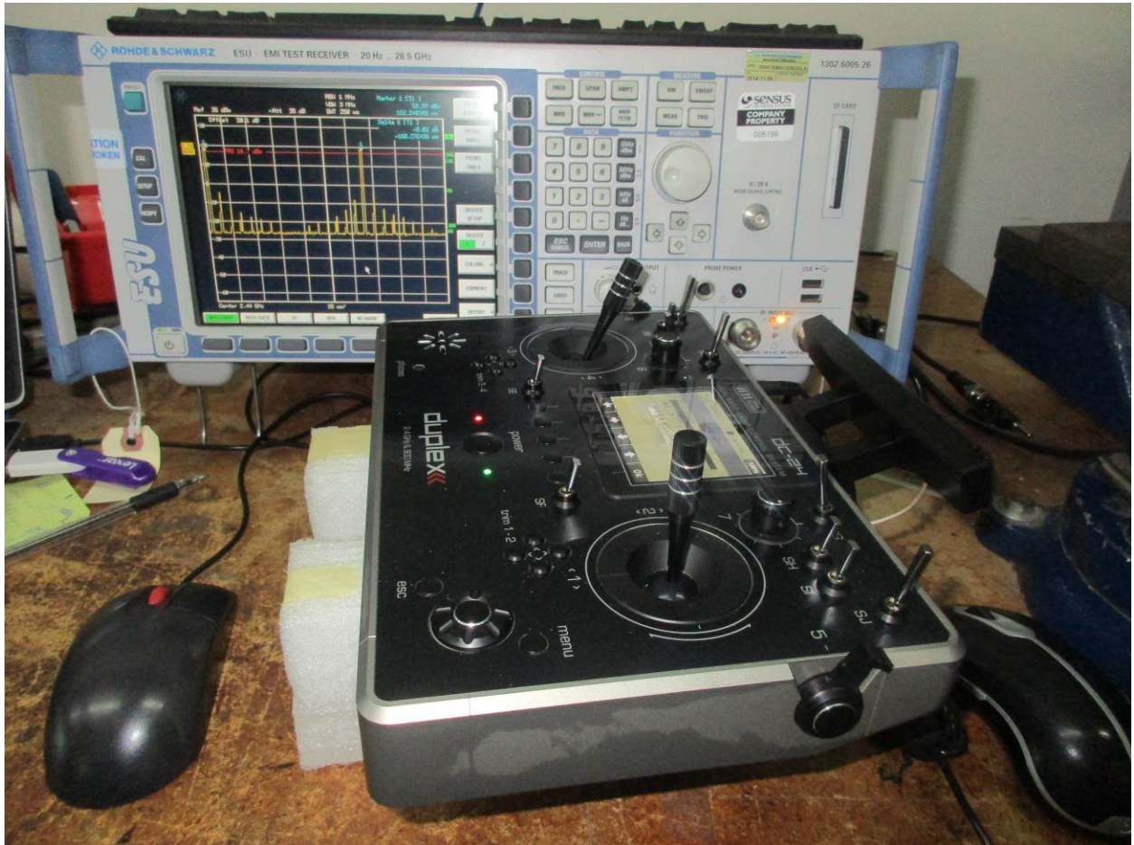
Figure 15: RF Conducted Emissions
