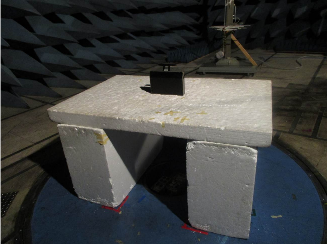
Figure 4: Radiated Emissions – Back View – 200 MHz – 1 GHz (900 MHz)
