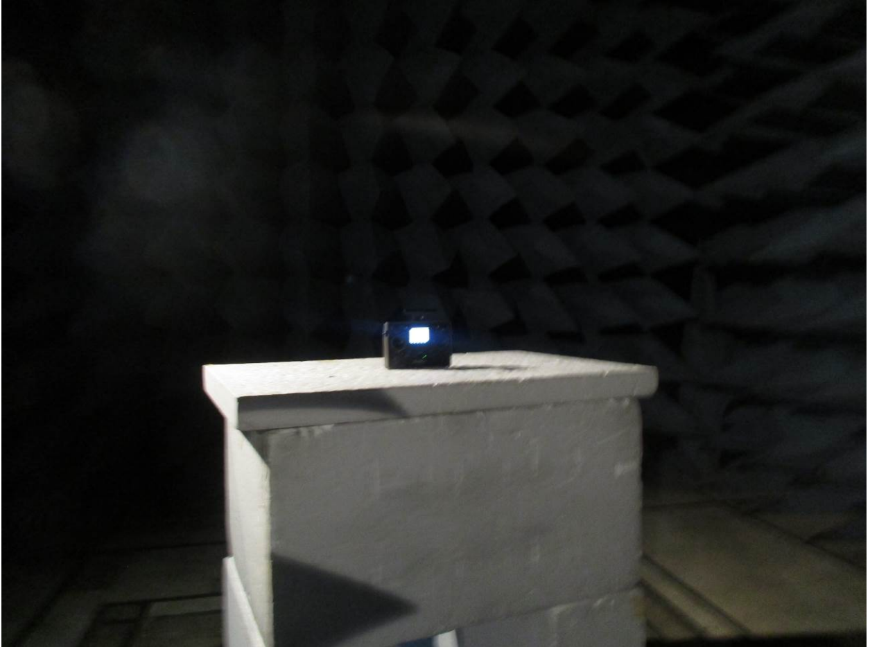
Figure 5: Radiated Emissions – Front View – Above 1 GHz (900 MHz, 2.4 GHz (AP1, AS1, AS2 Band Edge))
