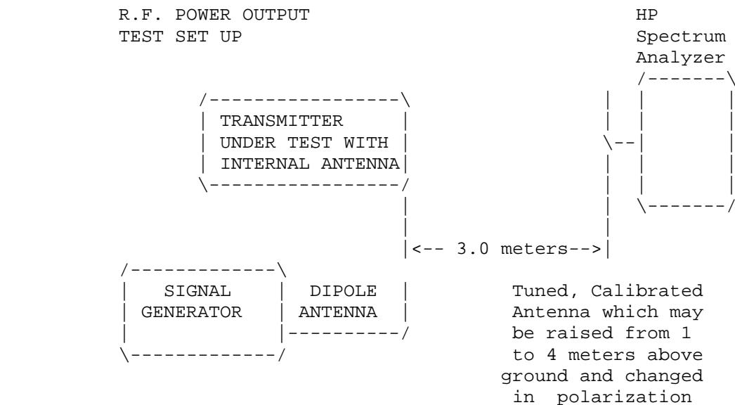
Equipment placed 1 meter above ground
