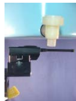
Face-held SAR Test Setup with 2.5cm spacing
