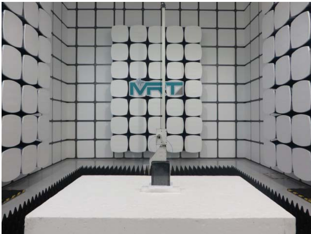
Description: Radiated Emission Test Setup for 18GHz ~ 40GHz
