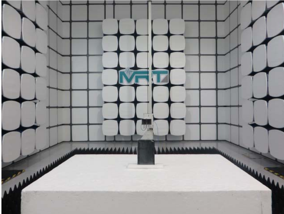
Description: Radiated Emission Test Setup for 18GHz ~ 40GHz
