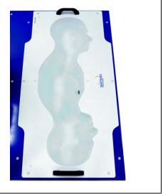
The bottom plate contains three pair of bolts for locking the device holder. The device holder positions are adjusted to the standard measurement positions in the three sections. A white cover is provided to tap the phantom during off-periods to prevent water evaporation and changes in the liquid parameters. On the phantom top, three reference markers are provided to identify the phantom position with respect to the robot.
